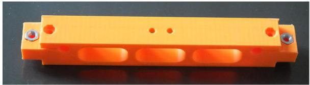
All m4 nuts in the design are nyloc with the exception of 4 full-nuts used in the bed supports in the positions shown.
