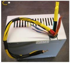
Identify all the 12V (yellow wires) at the ATX (large) connector and cut them as
