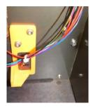
Now attach the PSU to the frame using 2off m4x20mm screws. Check that the back corner of the PSU is seated correctly in the bracket which you fitted at the same time as the Z-axis. Also
