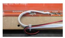
At this point you can insulate the bottom of the heated bed. If you are only going to print PLA then this is not necessary but if you are going to print ABS then it will help the bed reach and maintain the higher temperature needed to prevent the ABS from warping. PLA needs a bed temperature of around 60°C, ABS needs a temperature of around 105°C. Using the template provided cut out the insulator from corrugated cardboard and then
