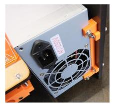
ensure that the wires for the Y-Endstop, Y-Motor and Z-Motor pass behind the power supply, secure them together with a cable-tie to ensure they stay in place.
