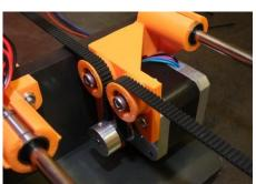
Take the GT2 belt left over from the X-axis. Pass it around the y-motor pulley and over the plastic pulleys. Secure each end in the clamps on the bed supports. If necessary adjust the belt tension by slackening the motor mount screws and pulling the motor downwards, before re-tightening. Trim off the excess belt.
