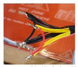
close to the connector as possible. Identify the 12V (yellow wires) at the CPU and Auxillary (all the other) connectors and cut them to the same length as the ones removed from the ATX Connector. Cut 10mm of insulation from the end of the wires. Take a short length of red wire cut from one of the other leads and
