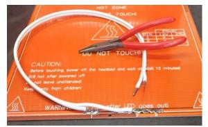
Strip the ends of the 500mm long 1.5mm^2 bed power cable and solder them to the bed heater as shown. Ensure that the PCB tracks (you can feel / see them, the other side is flat) are uppermost. Also ensure that when attaching the wires to the board that no solder flows onto the other side, this needs to be flat. Strip 5mm of insulation from the free ends and tin the copper core. At this point it is worth checking
