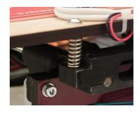
Attach the bed assembly to the bed supports using M4x35 button head screws with plain washers under their heads and 20mm springs between the bed assembly and the bed supports.
