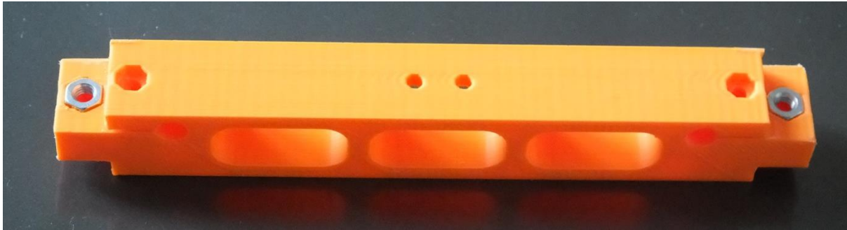
bed support showing plain nut positions
